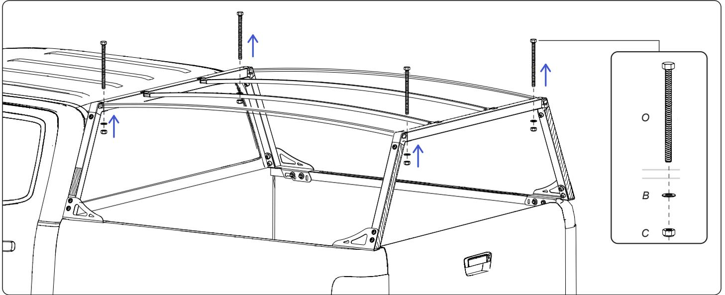
Then place the canopy cover on the frame and locate the holes in tube to be poked in through the cover. Slide front of cover through rope track from one side.
