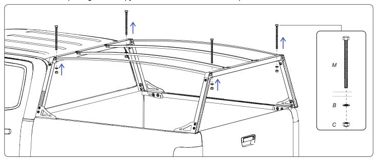
Then place the canopy cover on the frame and locate the holes in tube to be poked in through the cover.
