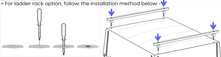
> Locate the holes on the corners of the top frame and carefully punch holes through them with a phillips head screw driver. Install ladder racks using the order below.
