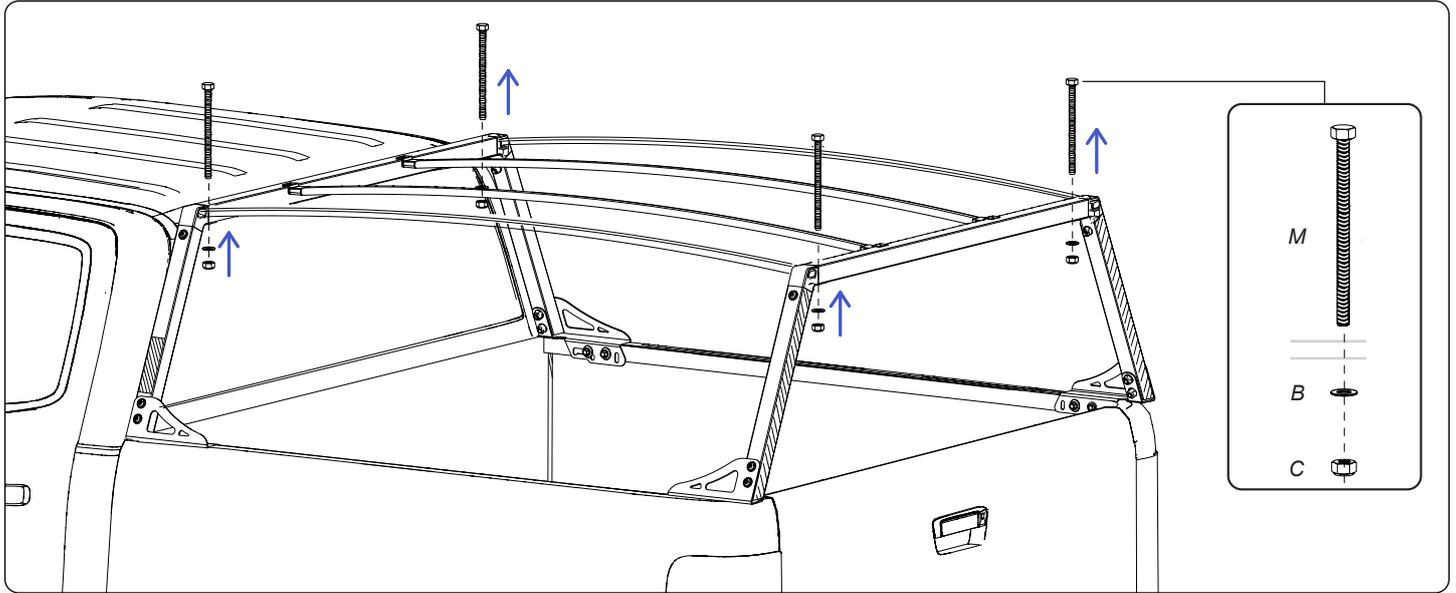
Then place the canopy cover on the frame and locate the holes in tube to be poked in through the cover.
