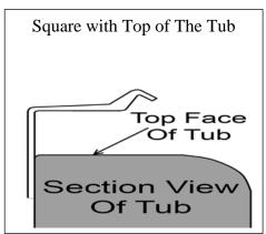
(c) Drill through those locations into tub, using 4.5 drill bit. Then rivet into 50mm, 350mm, 920mm and 1170mm.
