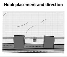
The plastic clips on the internal shock cord can be hooked into the aluminium extrusions so that the cover can still be secured with larger loads in the tub.
