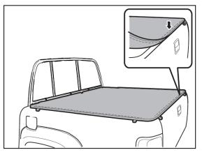
13. Clip the driver's side of the cover onto the driver's side extrusion then attach the passenger side of the cover using the pull loops in the corners to help stretch the cover.
