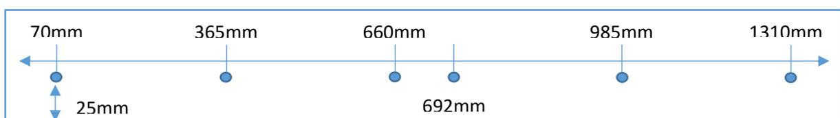
**IMPORTANT:** Keep ALL Rails flush with top of the Tub Walls and Tailgate while drilling.
