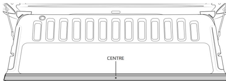
b. Measure and mark all 5 points on the aluminium rail (*see Figure 9*) then drill out all 5 using a 4mm drill bit. We recommend drilling just the aluminium rail in this step.
