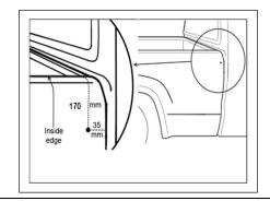
Measure down <u>155mm</u> from the inside edge of the tub, and forward <u>5mm</u> from the front outside edge of the tailight and mark.
