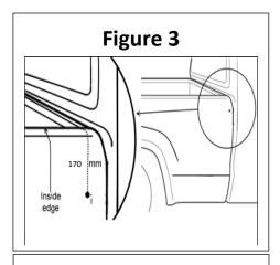
(b) Measure down <u>150mm</u> from the inside edge of the tub, in line with the Rear-Side Bunji and mark. *See Figure 4*
