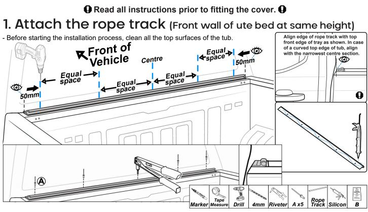
> Measure and centre align the rope track and place the track flush to the top front edge of the tub as shown above.
