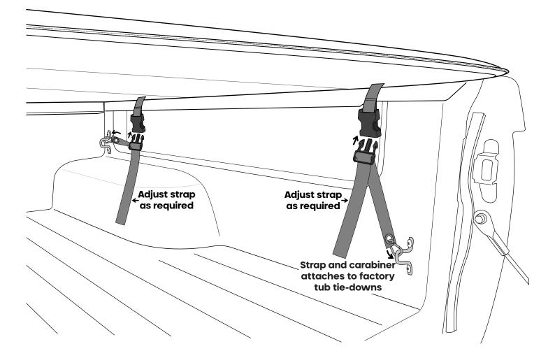
> Locate factory mounted tie-downs in tub and attach the carabiner with strap to them as shown above. Attach the buckles.
