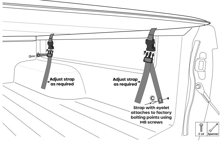
> Locate factory mounted bolting points in tub and attach the strap with the M8 screws  $\bigcirc$  provided. The screw goes through the strap's eyelet and into the bolting points. Tighten screws with 13mm spanner. Attach the buckles.
