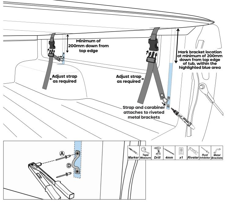
> Measure and mark the metal bracket **D** location to be drilled and riveted at a minimum of 200mm down from top edge of the tub. Keep the bracket location on the tub **in alignment with the buckles on the Ezy Fold cover**.
