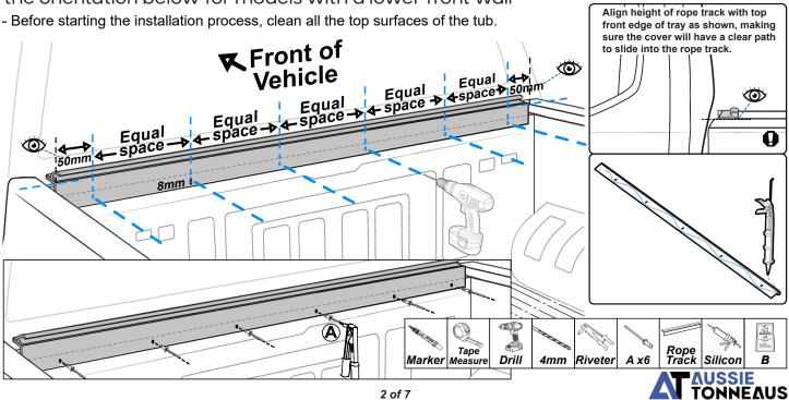
> Ensure the rope track is aligned at same height as the side walls of tub. Centre align the rope track and place the track flush against the front wall of the tub as shown.
